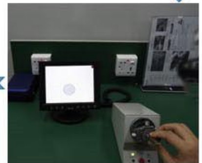
Cleaning end face
